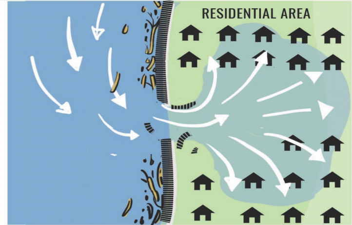
As a result, breaches in the wall become inevitable which could occur near many riverside residential areas of Laredo. These points of failure in the wall would be sites of catastrophic flooding.
